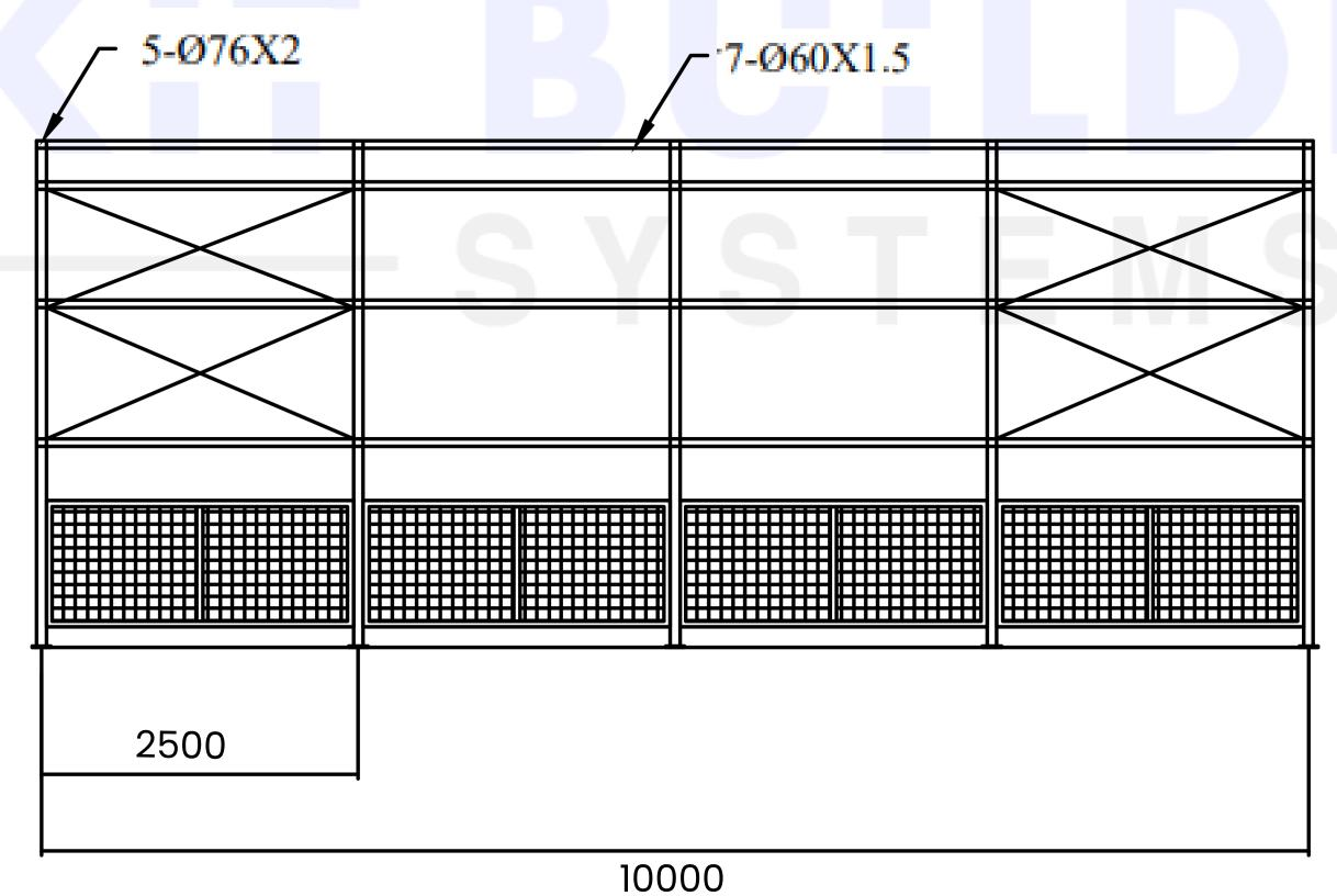
Opening/Shutter Size WxH: Arch Tube Thickness: Purling Tube Thickness: Covering: **Steel Frame:** Eave Height: CHS 3.848m x 4m PVC 610g/m2 | 76mm x 2mm | 60mm x 1.5mm | 1.5m | 4'9" 12'6"" x 13'1" 21.21oz/ft Single Truss 2.99" x 0.08" 2.36" x 0.06" Pedestrian door **ELEVATIONS** Quantity: N/A PAGE 1 OF 1 Size: N/A Material: N/A
